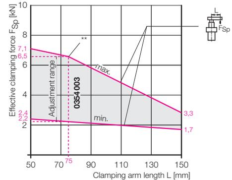
\*\* For clamping arm lengths > 75 mm, please observe the setting parameters permitted for the effective clamping force as specified in the operating instructions.
