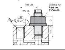
3. Connecting housing and lock nut
