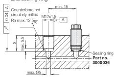
2. Screw-in thread and sealing nut
