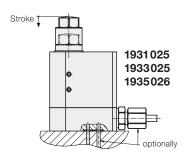
When loading the fixture, the support plunger is pushed back by the workpiece and contacts the workpiece by spring force. Then hydraulic locking can be effected. During unclamping the support plunger will be unlocked and moved forward by a little spring force when unloading the workpiece.
