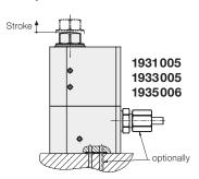
When pressurising the element, the support plunger moves forward with a light spring force against the workpiece. Then locking is automatically effected.
