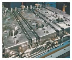
Swing sink clamps in a double-column press The tie rod is extended (swing position). Die positioning is made by lateral stops. Easy feeding of dies by hydraulic roller bars installed in the T-slots.
