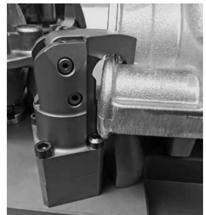
Clamping of a cast part with special clamping lever
