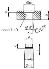
Clamping arm with contact bolt
