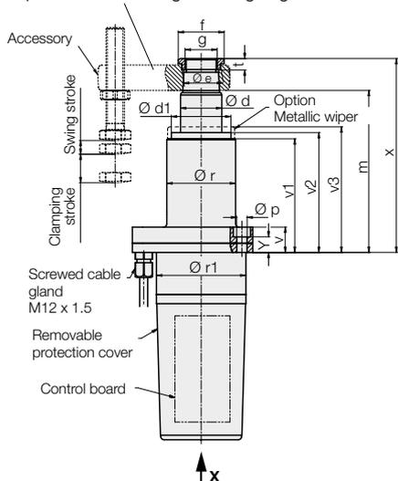
Clamping arm can be fixed in any desired position.
