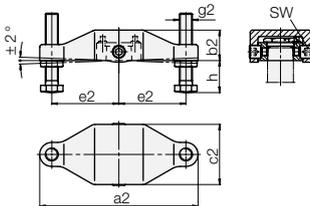
Carrier for double clamping arm 42CrV4 hardened and tempered
